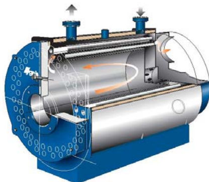
Figure 2: Two-pass reverse flue fire-tube hot water boiler
